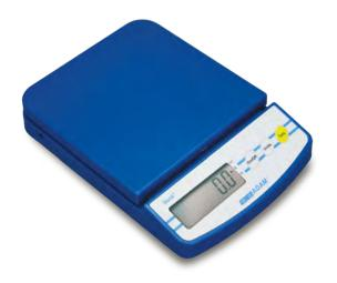
With a user-friendly, low-profile design, the Dune compact balance offers simple operation using just three buttons: on/off, unit, and tare. The portable Dune delivers reliable readings in the lab or field.
